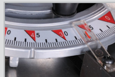
Set the cutting table to a precise angle
