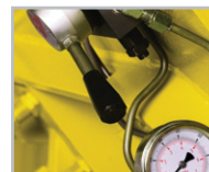
Hydraulic blade tensioning
