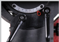
Angular cutting table up to 45°
