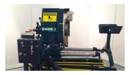
This is the world's only portable bevelling machine capable of servicing the smallest Rotary Shouldered Connections from NC26 (2 3/8" IF) or 2 3/8" regular up to one of the largest, 7 5/8" regular connections.
